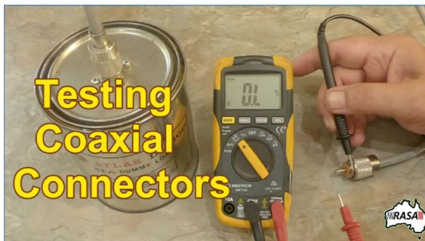
Coax connector Continuity testing – YouTube
