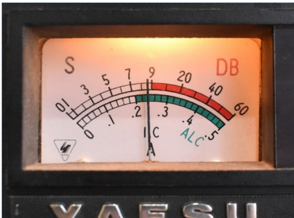
Above S-9 meters have a decibel scale indicating the number of decibels over S-9.
