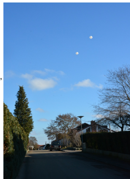
Fig 1. balloon antenna for 80m in 2el Yagi config; balloon height 55m.
